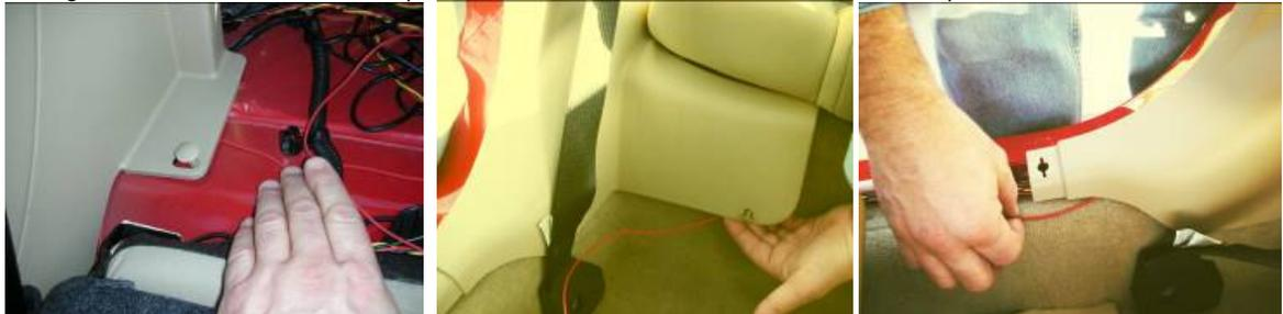
5. Remove the round plastic trim retainer below the back seat and near the carpet (passenger side) so Red power wire can be routed behind and to the scuff plate (threshold).
