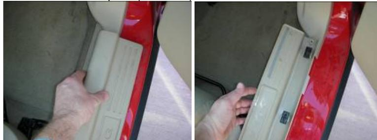
6. Remove the scuff plate (threshold) and continue Red power wire to passenger side kick panel. **NOTE: To remove the scuff plate all you have to do is pull up starting from one corner working your way to the other side.**
