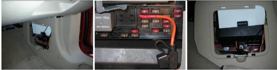
8. With fuse box cover removed. You will notice an unused fuse located closes to the Grey relay. Refer to picture. Plug the brass terminal from the Red power wire into the empty fuse slot that is closest to the Grey relay. Please refer to picture, if you plug into the other slot, the unit will not work because this slot has no power. Before installing the fuse cover you will need to cut a "V" or "U" shape notch in it to allow the Red power wire to pass through.
